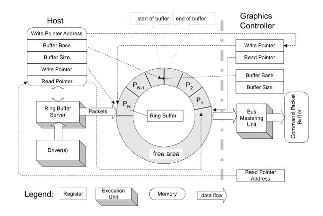
Figure: Ring Buffer and its Control Structure
