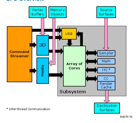
The subsystem consists of an array of *execution units* (*EUs*, sometimes referred to as an arrray of *cores*) along with a set of *shared functions* outside the EUs that the EUs leverage for I/O and for complex computations. Programmers access the subsystem via the 3D or Media pipelines.
