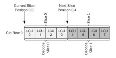
For error stream cases where the next slice position does not align itself with the last successfully decoded Ctb in the current slice, the HCP will conceal Ctbs from the last decoded Ctb in the current slice through to the last Ctb prior to the Ctb indicated by the next slice position. If the error occurs such that the current decoded Ctb cannot be decoded, the HCP will ensure that the current Ctb is written out
