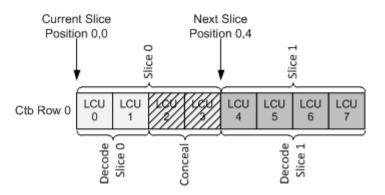
Since the host software removes overlapping slices, the next slice position will never be equal to or less than the current slice position.
