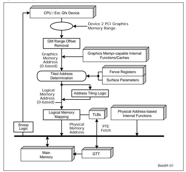
The remainder of this chapter describes the basic features of the graphics memory address pipeline, namely Address Tiling, Logical Address Mapping, and Physical Memory types and allocation considerations.
