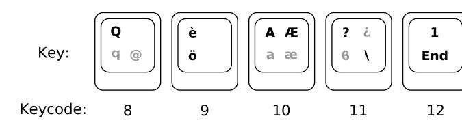
The core protocol represents this keyboard as a simple array with one row per key and four columns (the widest key, key 10, determines the width of the entire array).
