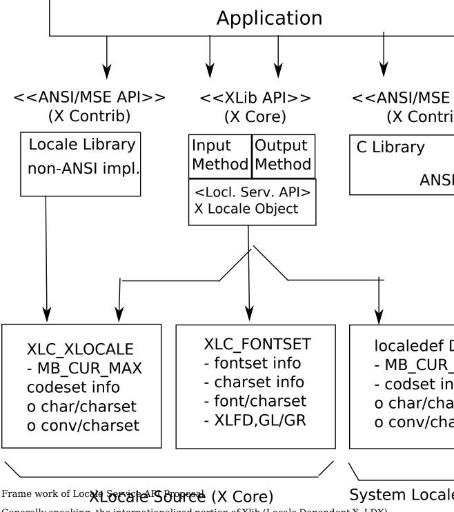
Generally speaking, the internationalized portion of Xlib (Locale Dependent X, LDX) consists of three objects; locale (LC) , input method (IM) and output method (OM). The LC provides a set of information that depends on user's language environment. The IM manages text inputing, and the OM manages text drawing. Both IM and OM highly depend on LC data.
