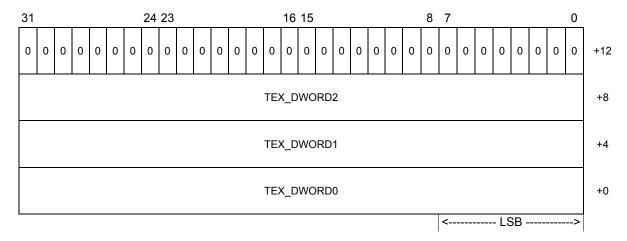
Figure 6.1 Microcode-Format 4-Tuple for Fetches Through a Texture Cache Clause
