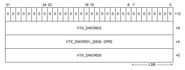
Figure 5.1 Microcode-Format 4-Tuple for Fetch Through a Vertex Cache Clause
