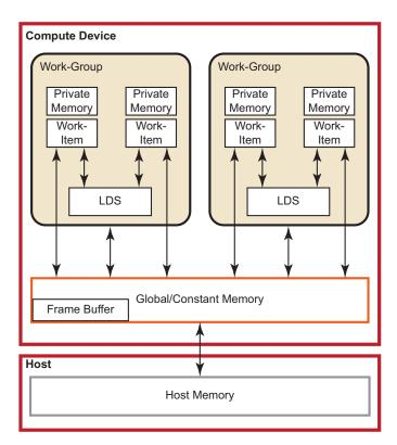
Figure 8.1 High-Level Memory Configuration
