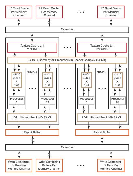
Figure 2.1 Shared Memory Hierarchy on the Evergreen Family of Stream Processors
