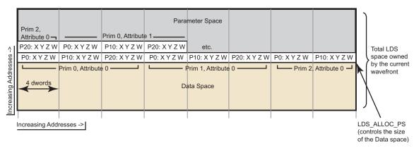
Figure 8.3 LDS Layout with Parameters and Data Share
