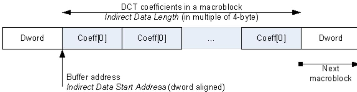
Each non-zero coefficient in the indirect data buffer is contained in a doubleword-size data structure consisting of the coefficient index, end of block (EOB) flag and the fixed-point coefficient value in 2's complement form. As shown in *Common Indirect IT-COEFF Data Structure*, index is the row major 'raster' index of the coefficient **within a transform block** (please note that it is not converted to 8x8 block basis). A coefficient is a 16-bit value in 2's complement.
