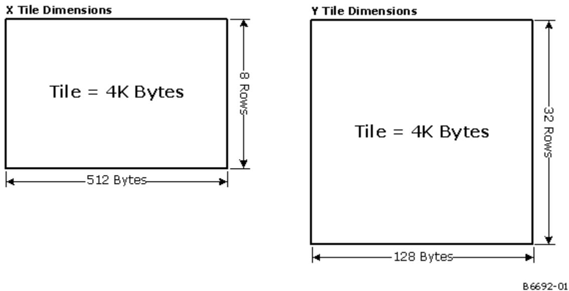
*The pitch of a tiled enclosing region must be an integral number of tile widths.* The 4KB tiles within a tiled region are stored sequentially in memory in row-major order.
