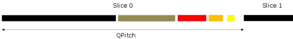
**Surface Pitch** is ignored for 1D surfaces. **Surface QPitch** specifies the distance in pixels between array slices. QPitch should allow at least enough space for any mips that may be present.
