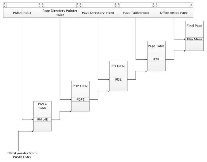
64bit (48b canonical) address requires 4-levels of page table format where the context carries a pointer to highest level page table (PML4 pointer) via PASID. The rest of the walk is normal page walk thru various levels.
