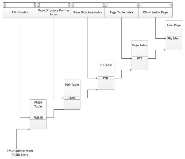
64bit (48b canonical) address requires 4-levels of page table format where the context carries a pointer to highest level page table (PML4 pointer) via PASID. The rest of the walk is normal page walk thru various levels.
