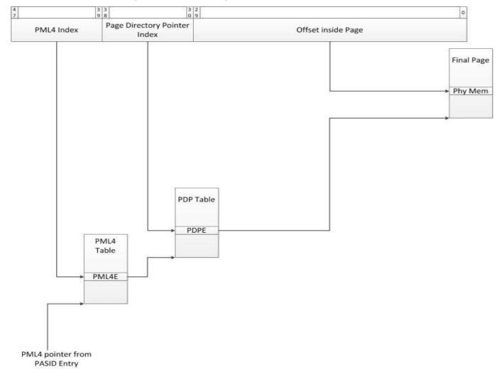
For the support for 1GB page size, the following mechanism is needed.
