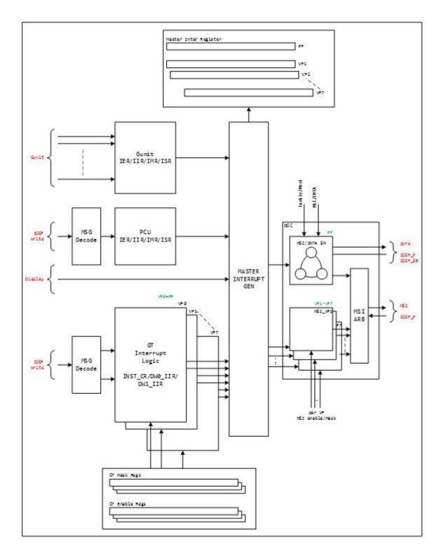
Interrupts to Host are delivered via a Master Interrupt Control Register. Graphics interrupts use 2 bits in the Master Interrupt Control Register. In addition, interrupt events from Display are also represented in
