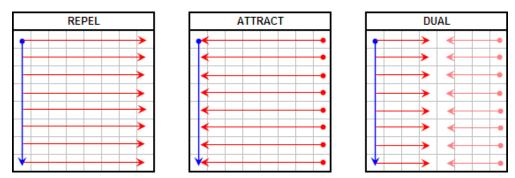
In Dual mode, the sequence will alternate between two half-walks such that every-other output would go to the same slice. This effect will produce a more balanced workload to two slices as shown in the example below where the color of the block represents which slice it was dispatched to. This is the walker's approach to fine-grained parallelism.
